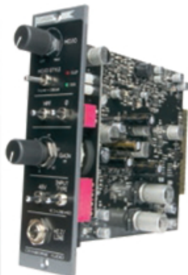
All-discrete circuitry with no transformers
